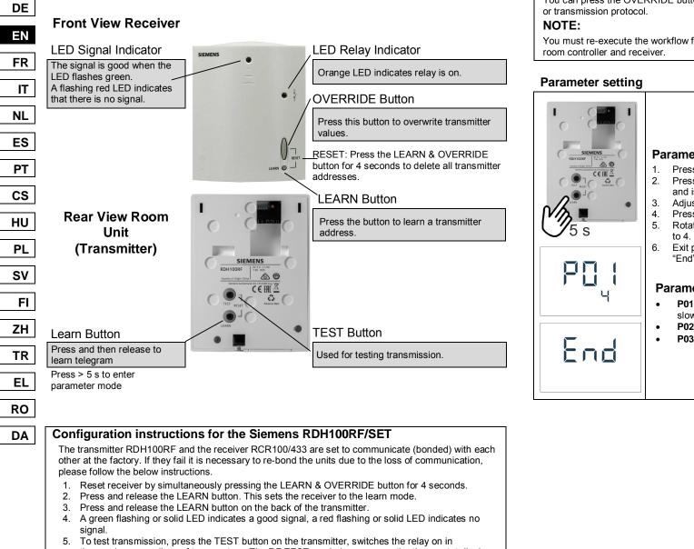
the receiver regardless of temperature. The RF TEST symbol appears on the thermostat display.An orange LED indicates that the relay is on.
